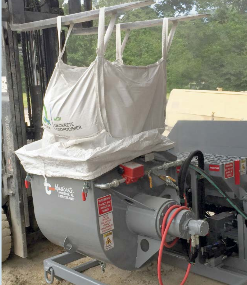
With OSHA getting ready to crack down on silica dust exposure, the problem of dust from products being poured into a mixer will only increase. The DustAway, which keeps dust from escaping, can be adapted to most large batch mixers.
