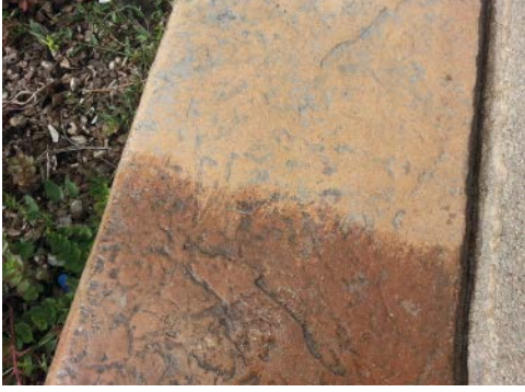
A new generation of color-enhancing penetrating sealers darkens the substrate without adding any gloss or creating potential issues associated with film-forming sealers.
