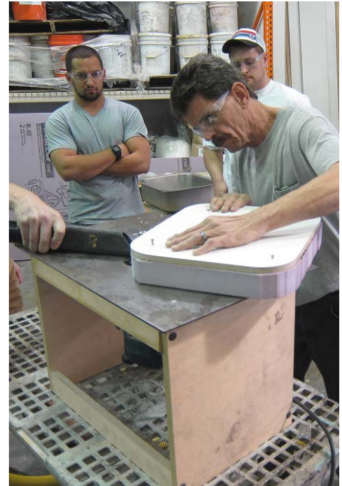
Here, class participants shape a foam sink knock-out on a router table to fit a wooden sink-hole template.
