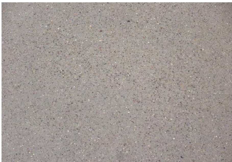
By adding larger aggregates to an overlay mix, it looks much more like concrete. Without aggregate, the materials have a plastic appearance.
