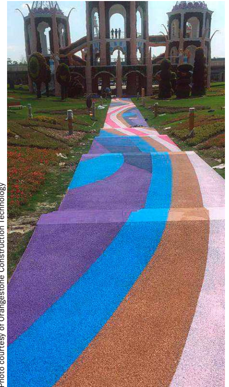
Integrally colored pervious concrete in multiple hues livens up walking paths at the Pujiang Country Park in Shanghai, China.
