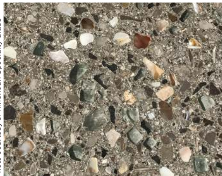
Seen here is an example of polished concrete with clear glass and mother of pearl aggregate.
