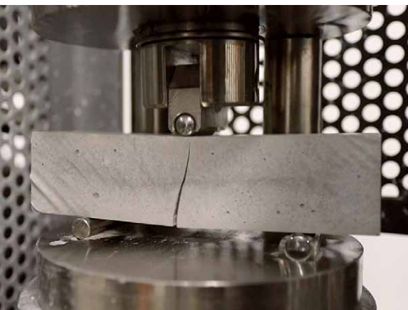
The downward force from the top causes the bottom of the prism to fail in tension during this ASTM C348 Test performed at the CTS laboratory.
