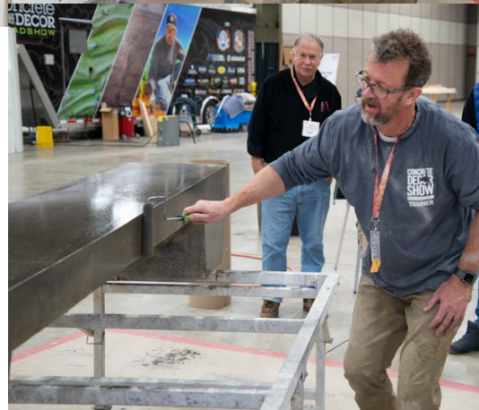
Artisan Jake Brady explains the benefits of his GFRC mix ( above ) and applies a high-gloss sealer ( right ).
