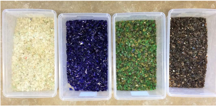
Clear, blue, green and amber glass aggregates are sorted by color before using them in concrete.
