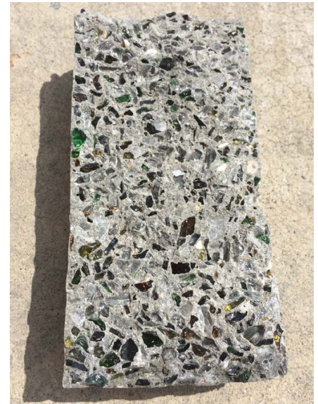
The sample seen here contains 100% recycled glass aggregate.
