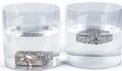
Ultra-lightweight concrete made with expanded glass floats in water.
